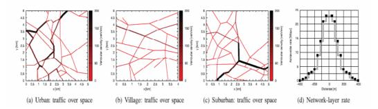
Figure 3. Road layout in the (a) urban, (b) village, and (c) suburban scenarios, and achievable network-layer rate characterization as a function of distance (d).
