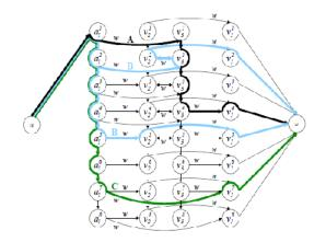
Figure 1. A sample DNTG, with one Access point A and three vehicles v1, v2 & v3, the vehicle (v1) is a downloader while the others (v2, v3) can act as relays. In the above graph, we show up paths that are agent of the carry and-forward (A), connected forwarding (B), and direct transfer (C) paradigms.
