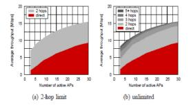
Figure4. Partition of the average downloader throughput with respect to the number of relays between AP and downloader (Max-flow deployment strategy)
