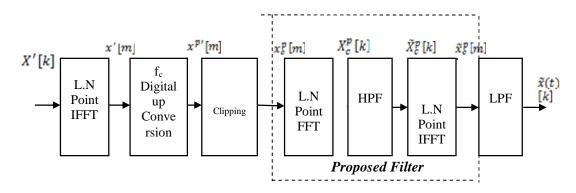
Figure 4. Block Diagram of Proposed Clipping & Filtering Scheme.
