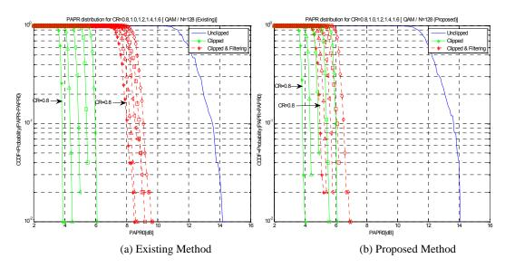
Figure 6. PAPR Distribution for CR=0.8,1.0,1.2,1.4,1.6 [QAM and N=128]
