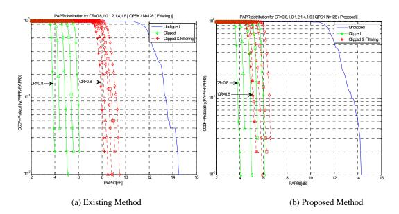
Figure 5. PAPR Distribution for CR=0.8,1.0,1.2,1.4,1.6 [QPSK and N=128]
