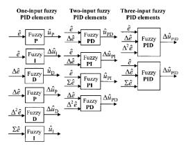
Figure 5. Fuzzy PID structural elements.
