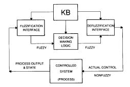
Figure 3. Basic configuration of fuzzy logic controller (FLC).
