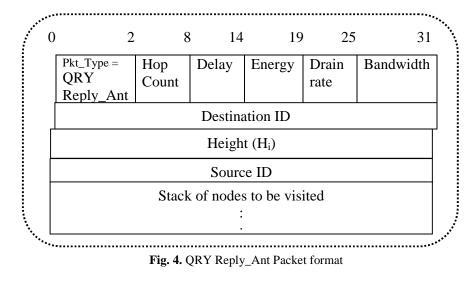
Fig. 4. QRY Reply\_Ant Packet format
