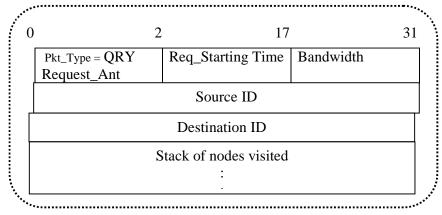
Fig. 3. QRY Request\_Ant Packet format
