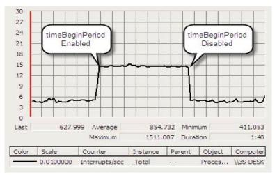
Figure 4. Effect of enabling and disabling timeBeginPeriod on performance.
