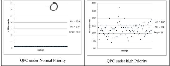
Figure 8. Performance of timers on windows XP using the same PC.
