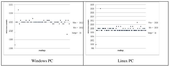
Figure 9. Performance of RealTime timers on Windows and Linux respectively.
