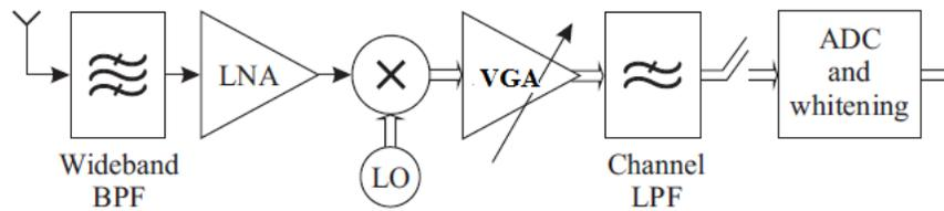
Figure 1. CR Receiver Diagram
