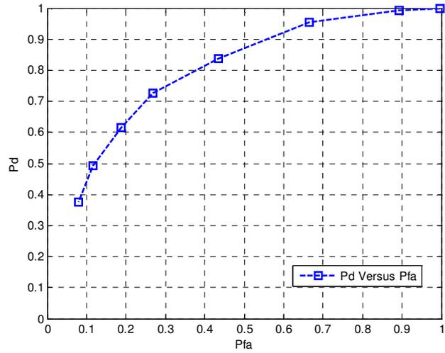
Figure 3. ROC curve with SNR=10dB for m=8 and n=50
