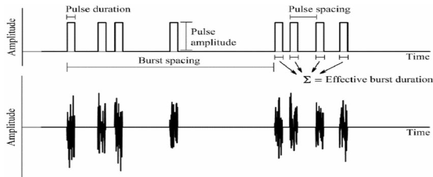
Figure 2. Impulsive Noise waveform
