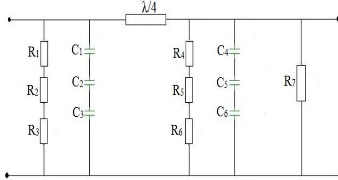
Fig. 3: Equivalent circuit of the Linearizer
