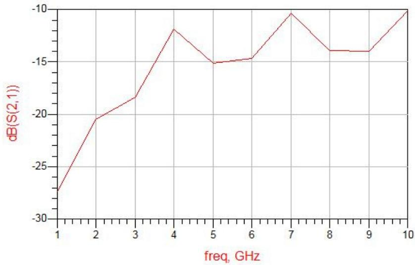
Fig. 10:  $|S_{21}|$  at 1.6 GHz of circuit using 5 Schottky diodes
