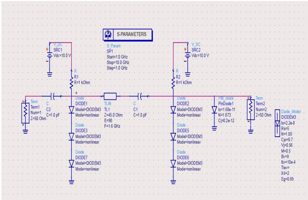
Fig. 5: ADS simulation screenshot for the simulation of three diodes in series
