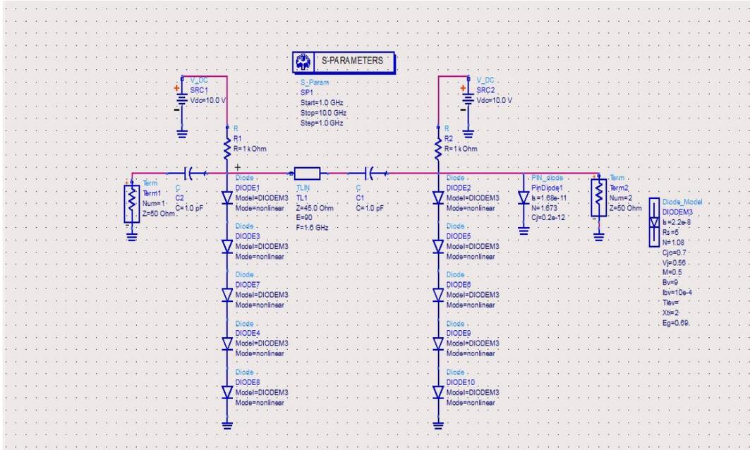
Fig. 7: ADS simulation screenshot for the simulation of five diodes in series
