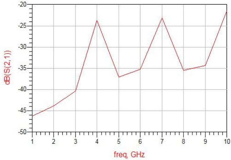
Fig. 9:  $|S_{21}|$  at 1.6 GHz of circuit using one Schottky diode
