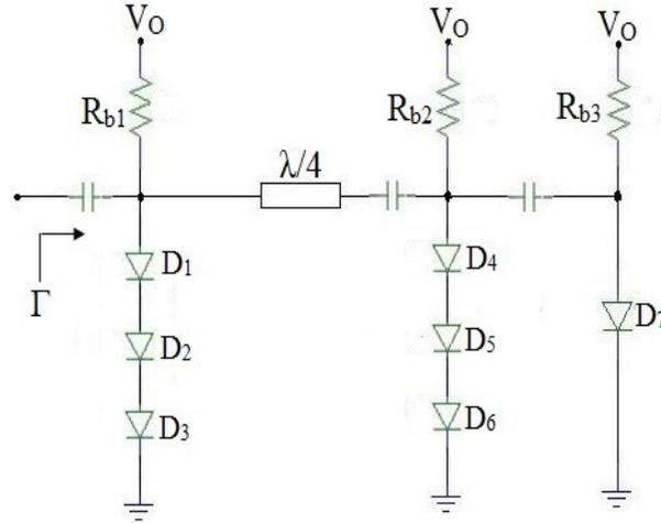
Fig. 2: Schematic Diagram of the circuit configuration L
