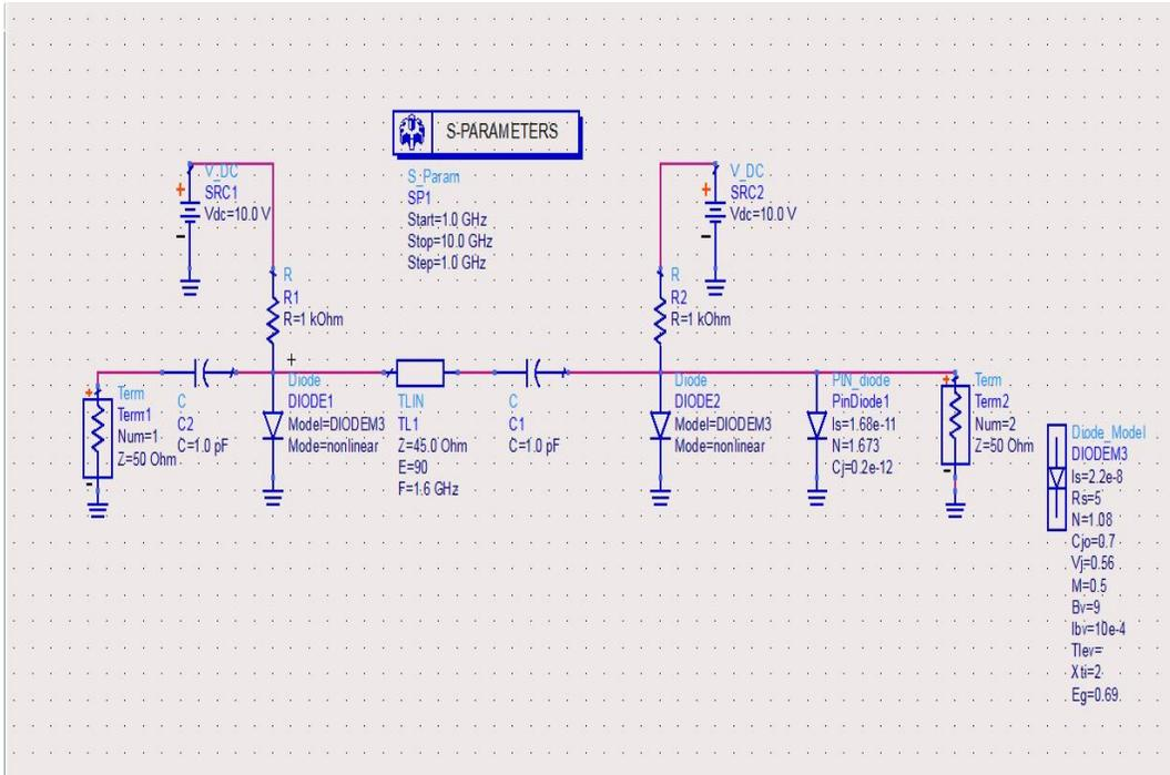
Fig. 6: ADS simulation screenshot for the simulation of one diode
