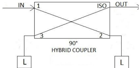
Fig. 1: Block diagram of the quadrature hybrid coupler
