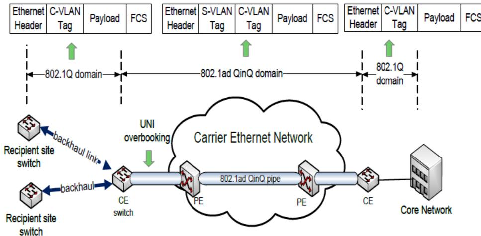
Figure 2. Q-in-Q Tunneling Carrier Backhaul Architecture
