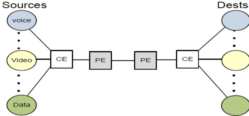
Figure 5. Dumbbell Topology for Network Simulation
