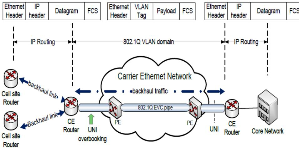
Figure 3. Cross-layer backhaul architecture
