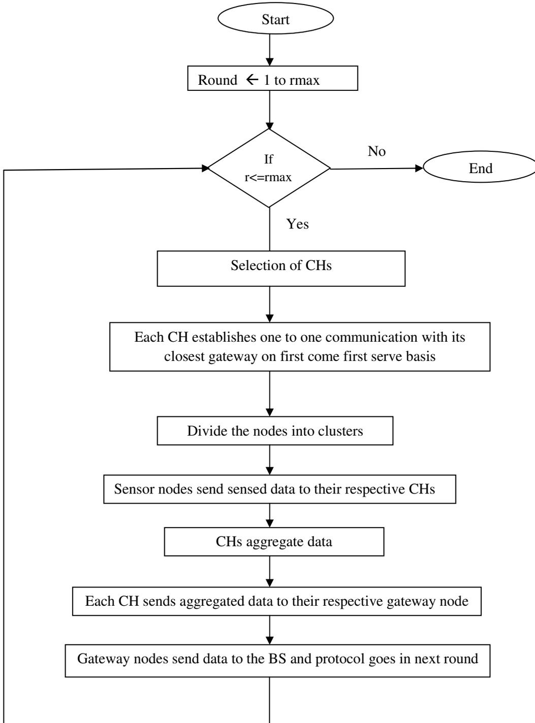
Figure 2. Flow Chart of Proposed Algorithm
