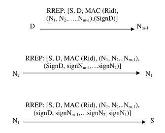
Figure 3: Route Reply Process
