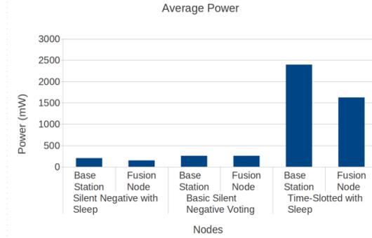
Figure 12: Average power consumption for Mica2
