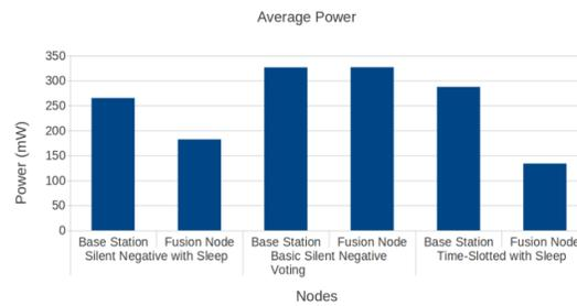
Figure 4: Average power consumption for TelosB
