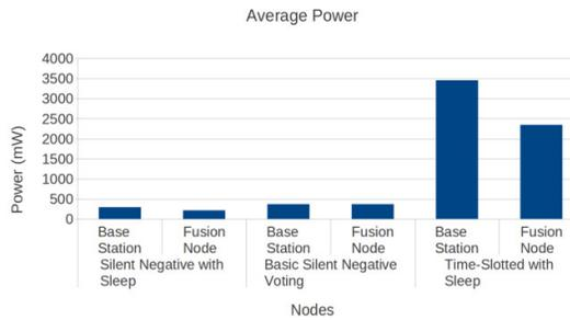
Figure 14: Average power consumption for TelosB
