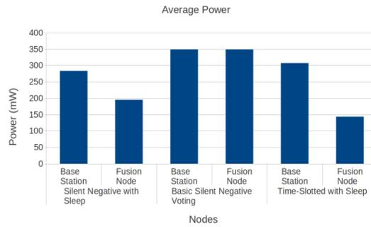
Figure 3: Average power consumption for MicaZ
