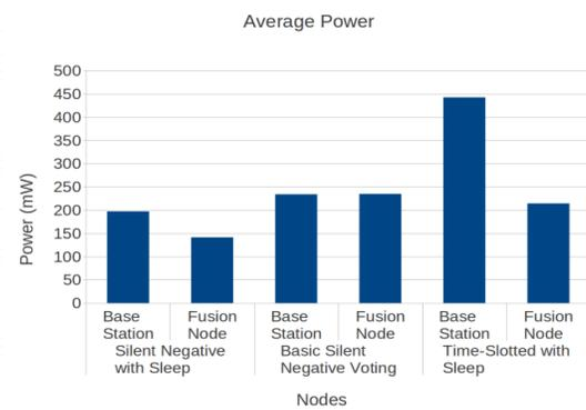
Figure 7: Average power consumption for Mica2
