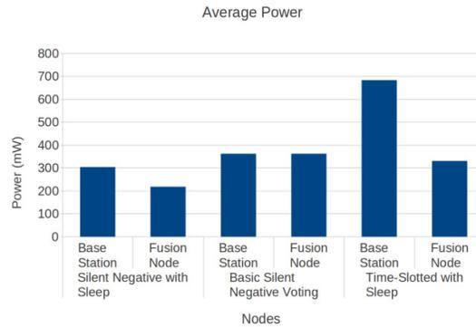
Figure 9: Average power consumption for TelosB
