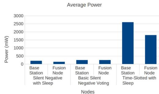
Figure 11: Average power consumption for TI CC1100
