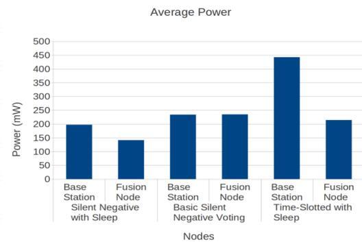
Figure 8: Average power consumption for MicaZ
