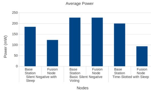
Figure 2: Average power consumption for Mica2
