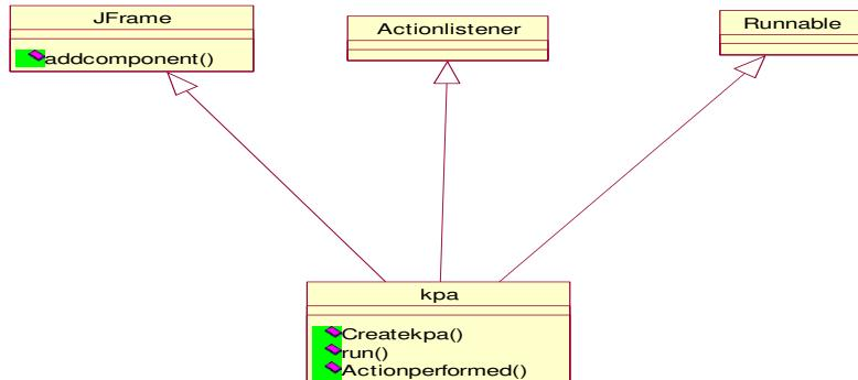
Figure 4: Class diagram for KPA
