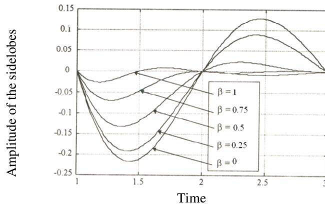
Figure 12: Sidelobes of the root-raised cosine pulse versus time for some  $\beta$ .
