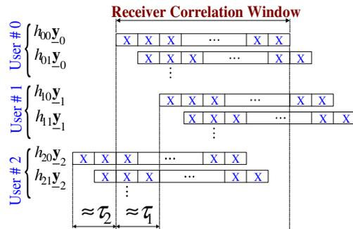
Figure 7: The users frame arrival at the base station receiver
