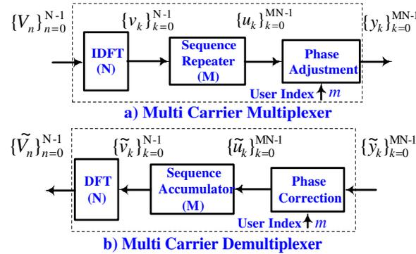
Figure 5: Reduced complexity multi carrier multiplexer (a) and demultiplexer (b).
