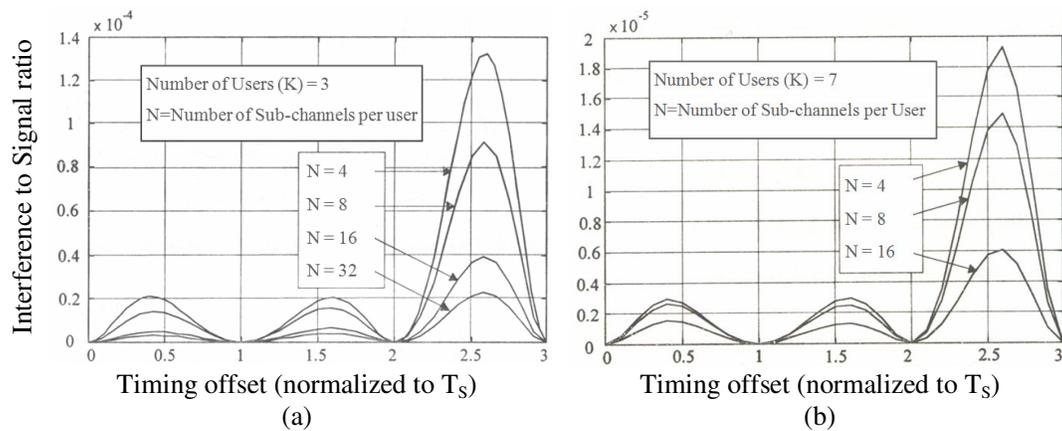
Figure 13: Interference to signal ratio versus time offset for some DFT size ( $KN$ ) when only one users has nonzero time offset,  $\beta = 0.25$ .
