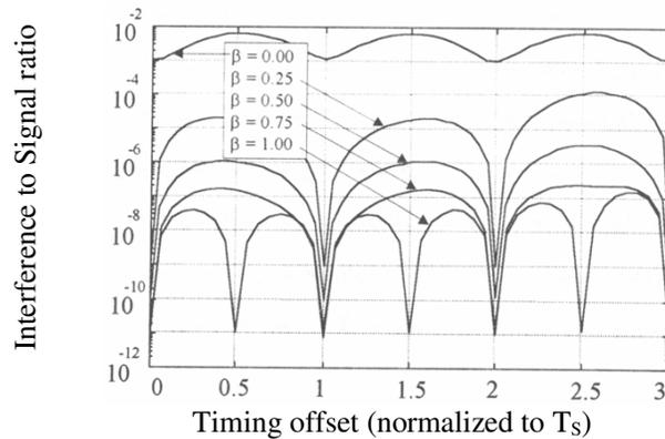
Figure 11: Interference to signal ratio versus time offset for some  $\beta$  ( $N=4$ ,  $K=3$ ).
