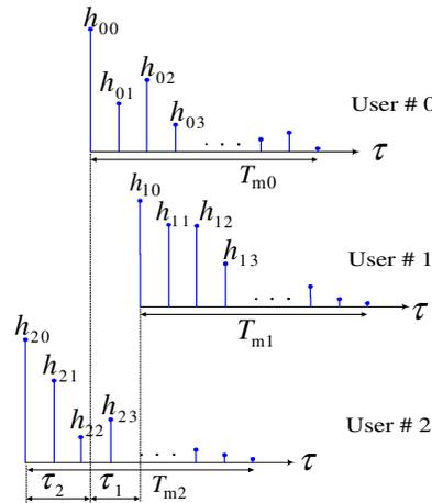
Figure 6: Relative propagation delays of the users sharing the same bandwidth
