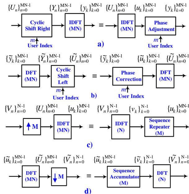
Figure 4: Equivalent discrete operations
