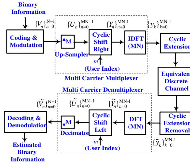
Figure 3: The straightforward digital implementation of interference tolerant OFDM
