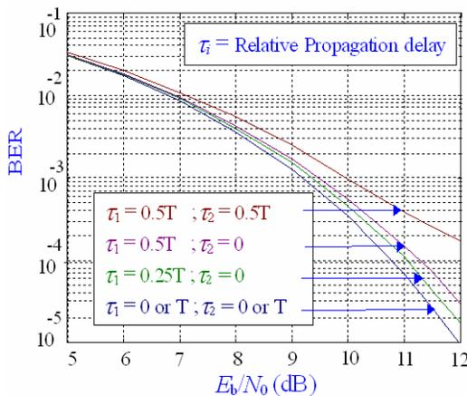
Figure 8: Performance comparison for various propagation delays over AWGN channel.
