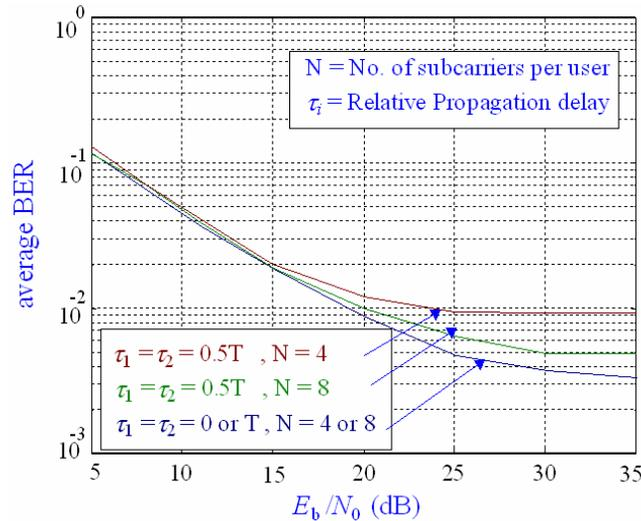
Figure 10: Worst case performance comparison for various numbers of sub-carriers per user over a Rayleigh fading channel.
