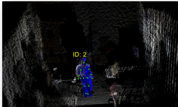
Figure 8. Labeled skeleton and associated joints obtained from the combination of 5 cameras information.
