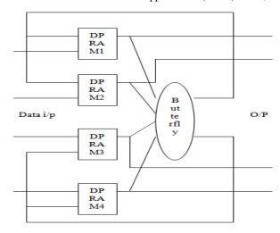
Figure 2. Dual memory (pair) architecture
