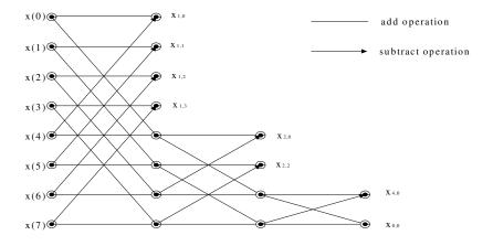
Figure 4. Figure showing the addition part of the 8-point paired transform based DFT
