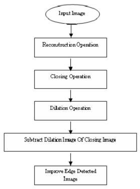
Fig.4.Flow chart of purposed algorithm
