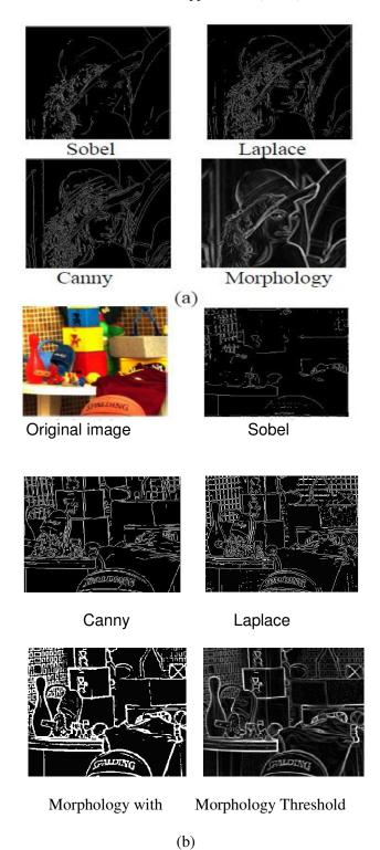
Fig.3. Comparison of traditional technique and morphology method.
