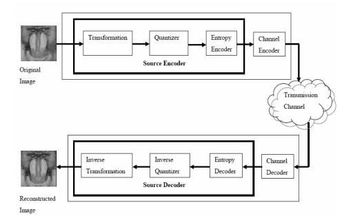
Figure:4 Basic block diagram for DCT conversion
