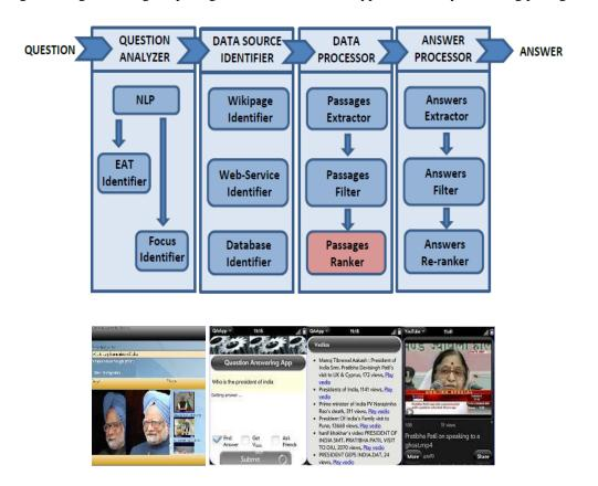
Figure 1 – Block Diagram of the QA System along with the screen shots of output on desktop and on mobile device simulator
