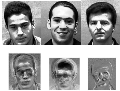
Figure 1. Row 1 shows some of the gray scale images used for training row 2 shows eigenfaces with significant eigenvectors.
