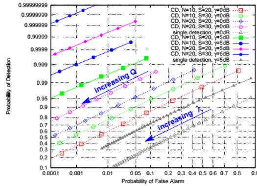
Figure 9. Primary user detection (  $\gamma$  - energy threshold parameter, Q- detection count threshold)
