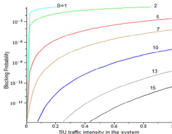
Figure 17. Blocking probabilities ( $P_B$ ) Against SU utilization in the system ( $\rho_2$ ). The Variation in  $P_B$  is depicted with different numbers of channels ( $S$ ), available with the system.
