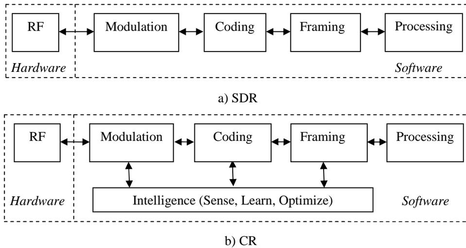
Figure 1. Block diagram contrasting (a) SDR and (b) Cognitive Radio
