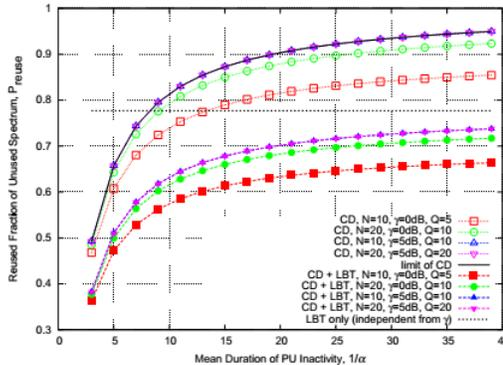
Figure 11. Efficiency of secondary reuse of spectrum unused by the PUs.
