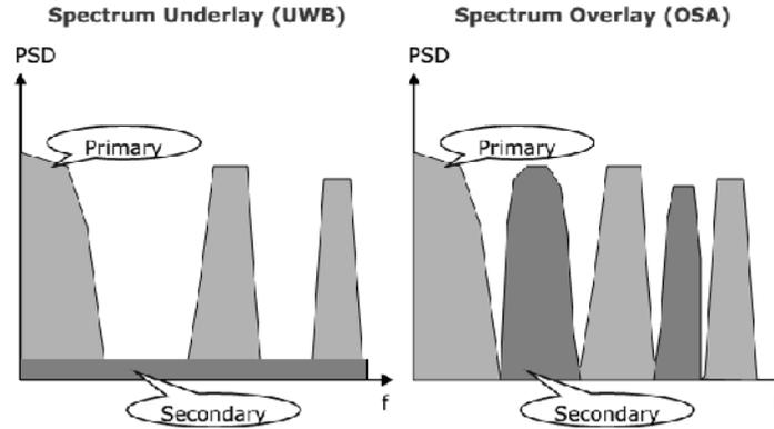
Figure 6. Spectrum overlay and underlay approaches
