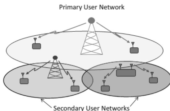
Figure 3. Coexistence of multiple primary and secondary user networks (homogeneous or heterogeneous)
