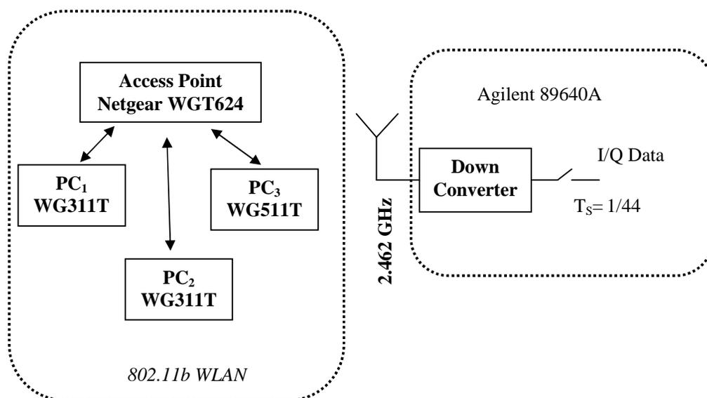
Figure 7. Measurement Setup
