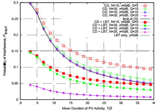
Figure 10. Probability of interference to the PU caused by CRs.
