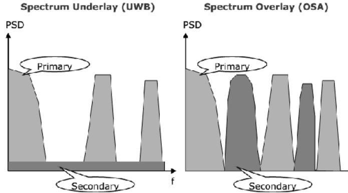
Figure 6. Spectrum overlay and underlay approaches
