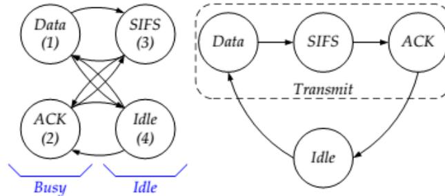
Figure 8. Proposed Markov model. The lumped model (with deterministic DATA SIFS ACK transitions is shown on the right).
