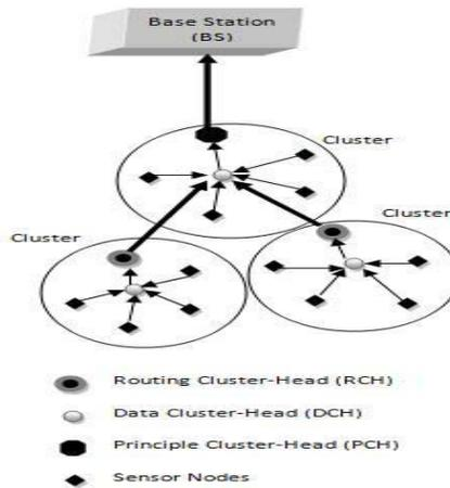
Fig 4: Clustering for RCH &amp; DCH selection
