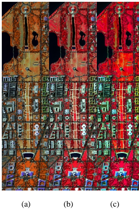
Figure 10. Fusion results. (a) Contourlet transform (CT). (b) Nonsubsampled contourlet transform (NSCT). (c) Contourlet transform with sharp frequency localization (CTSFL).
