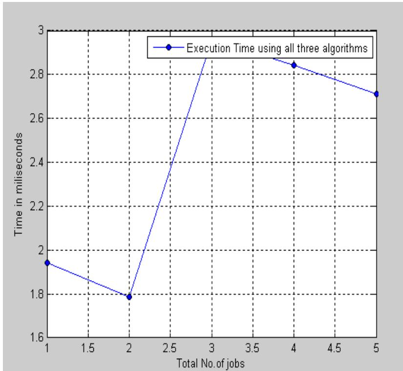
Figure 4. Execution time using all three algorithms (SJF, FIFO, RR)
