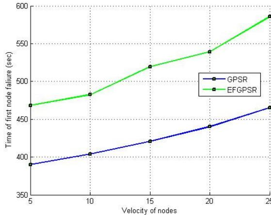
**Fig. 5.** 30 nodes with 15 s-d pairs having 50% greedy forwarding and 50% perimeter routing and 10% node both hard and soft faults
