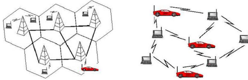
Figure 1. MANET with infrastructure (left side) and infrastructureless (right side) [2]
