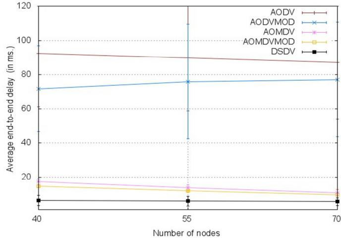
Figure 7. Results of End-to-end delay (in ms.)
