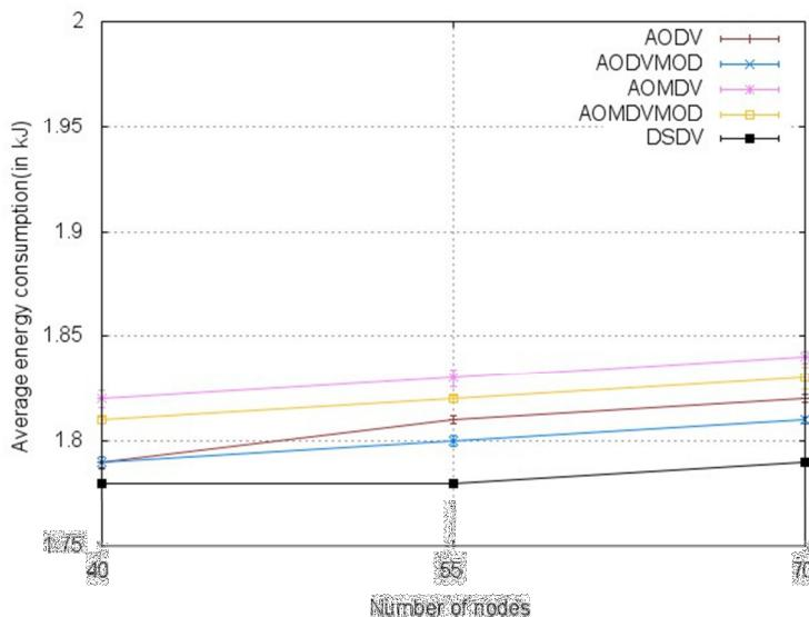
Figure 8. Results of Average Energy Consumption (in kJ.)
