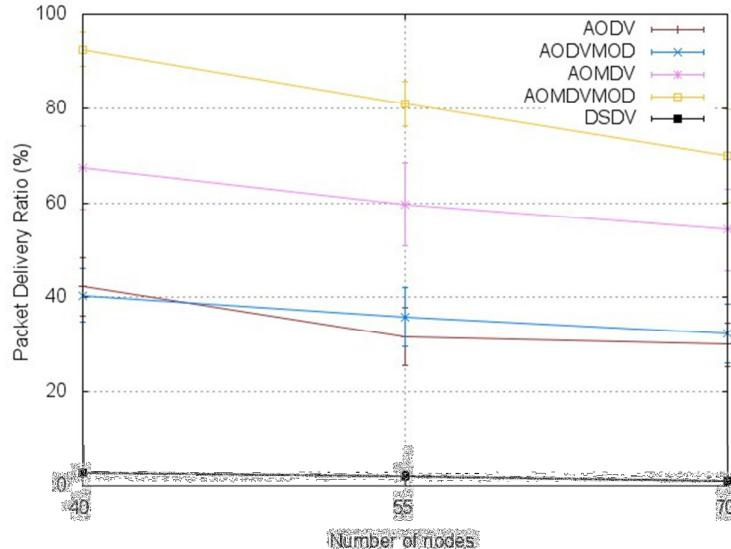
Figure 6. Results of Packet Delivery Ratio (%)
