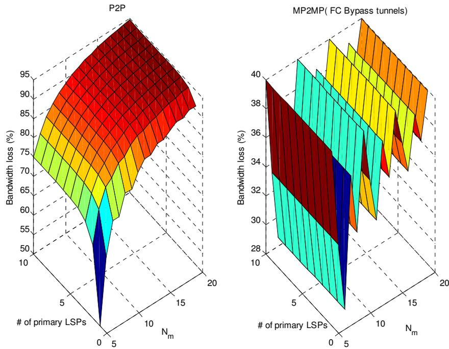
Figure 10 Bandwidth loss for  $N_l = \lfloor 0.6 \times N_m \rfloor$
