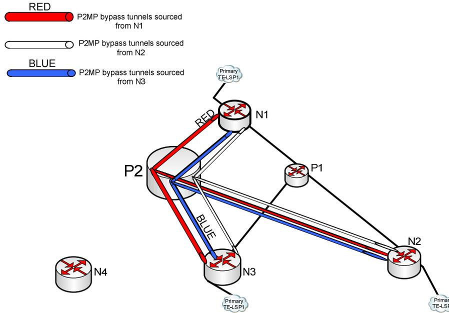
Figure 8 Protection using P2MP bypass tunnels
