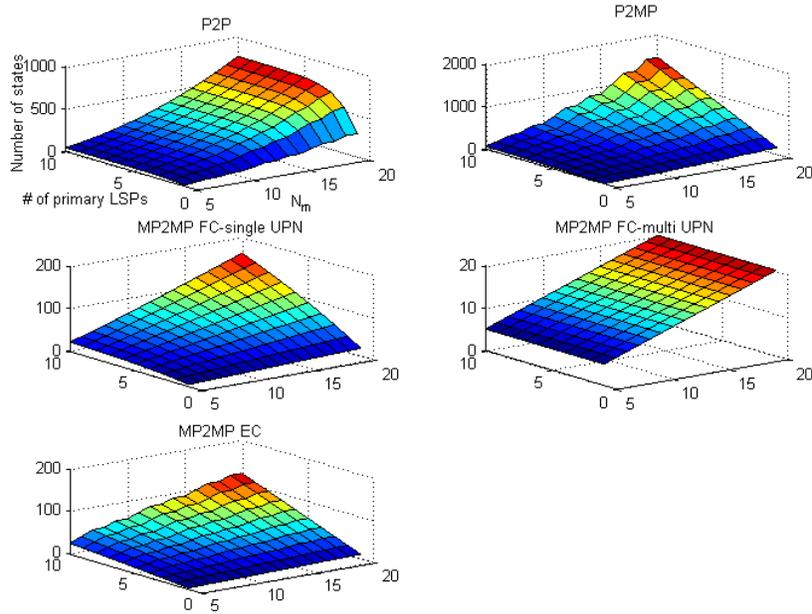
Figure 9 Number of states (z-axis) as function of  $N_m$  and  $l$  for  $N_l = \lfloor 0.6 \times N_m \rfloor$  (i.e. the integer part of  $0.6 \times N_m$ )
