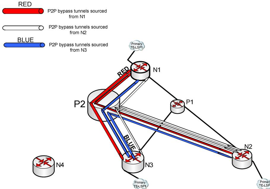
Figure 7 Protection using P2P bypass tunnels
