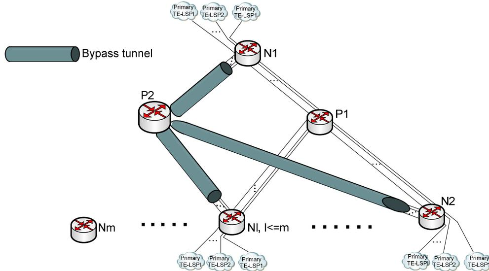
Figure 2 The bypass network is replaced by one node
