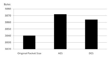
Figure 4. The space overheads of the IPSec for each security algorithm
