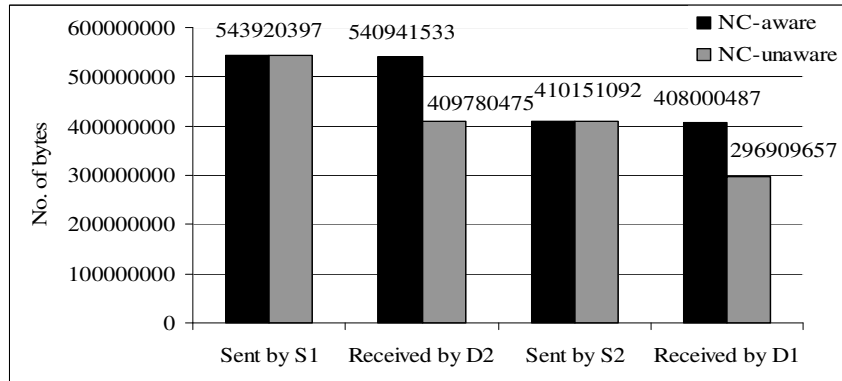
Figure 14. Number of bytes sent and received in the coded and uncoded case
