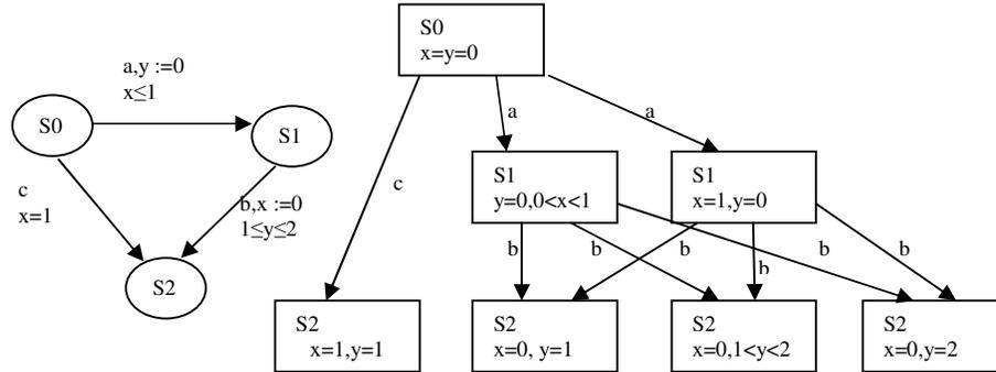
Figure 4. Timed automaton B and the associated region graph.
