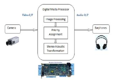
Figure 5. Hardware Implementation using DM642
